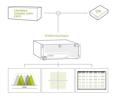
Deploy the DP-1000 to monitor, analyze and fix MAC-layer issues in real-time.
